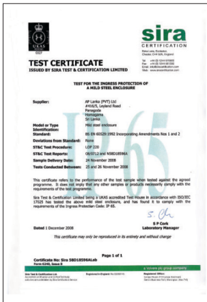
IP65, tested at UKAS accredited test lab in the UK
